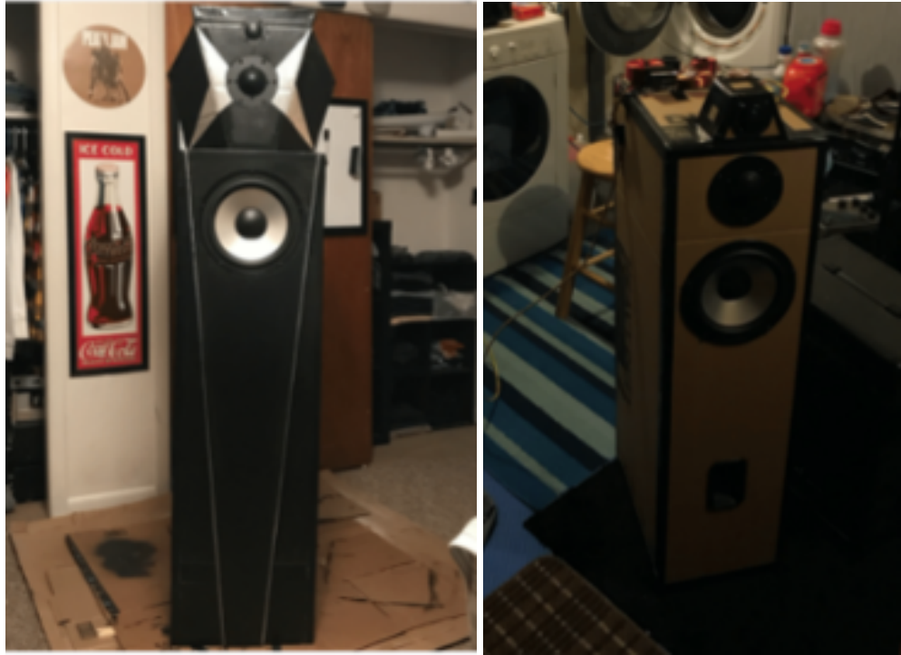
Figure 1: P1's first working prototype (left) versus final working prototype (right), showing adjustments to enclosure sizing and driver placements
